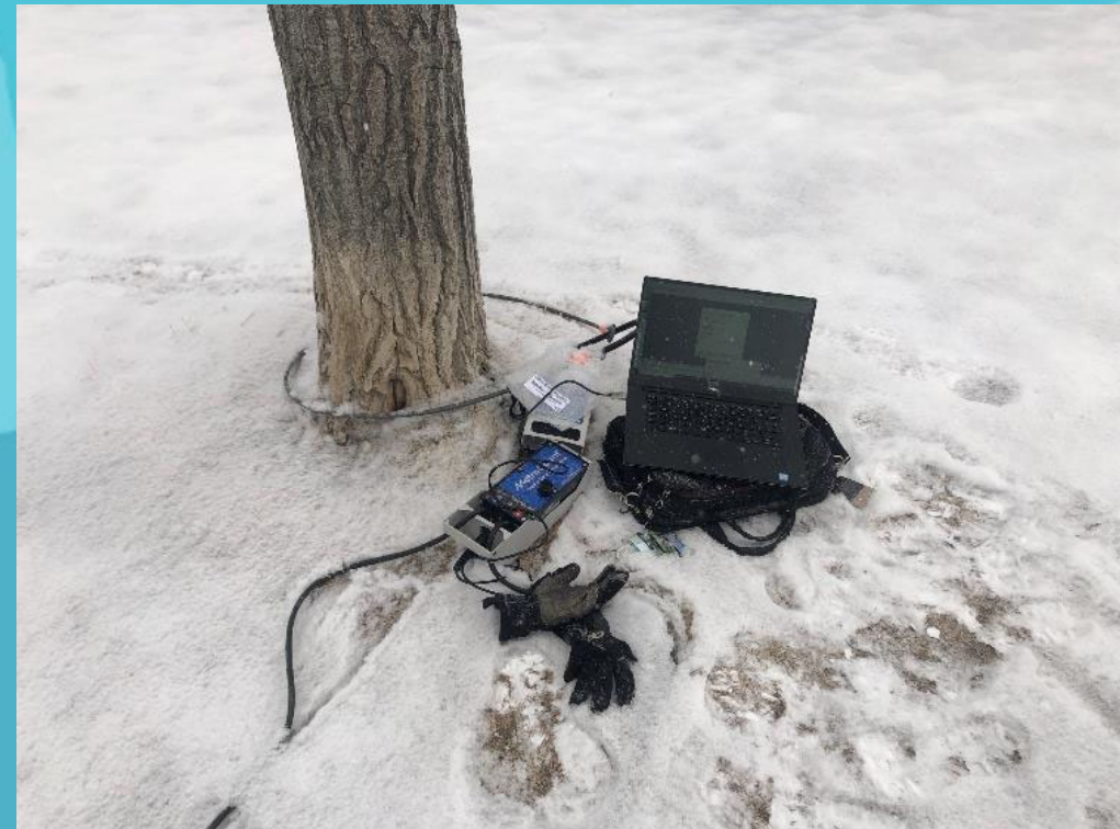
Metrocount RidePod BT with local storage, data retrieved at month end
